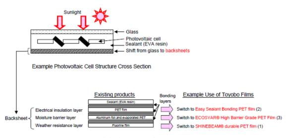
Example Backsheet Structure Cross Section
