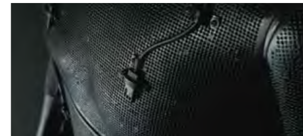
The TOM™ III has more than 200,000 sweating holes on its surface, and can measure temperature and humidity within clothing.
