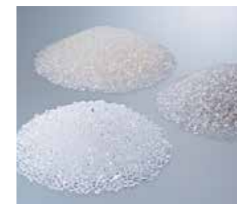
Polyester resins polymerized with different catalysts: TOYOBO GS Catalyst™ (front), antimony catalyst (right), titanium catalyst (back)
