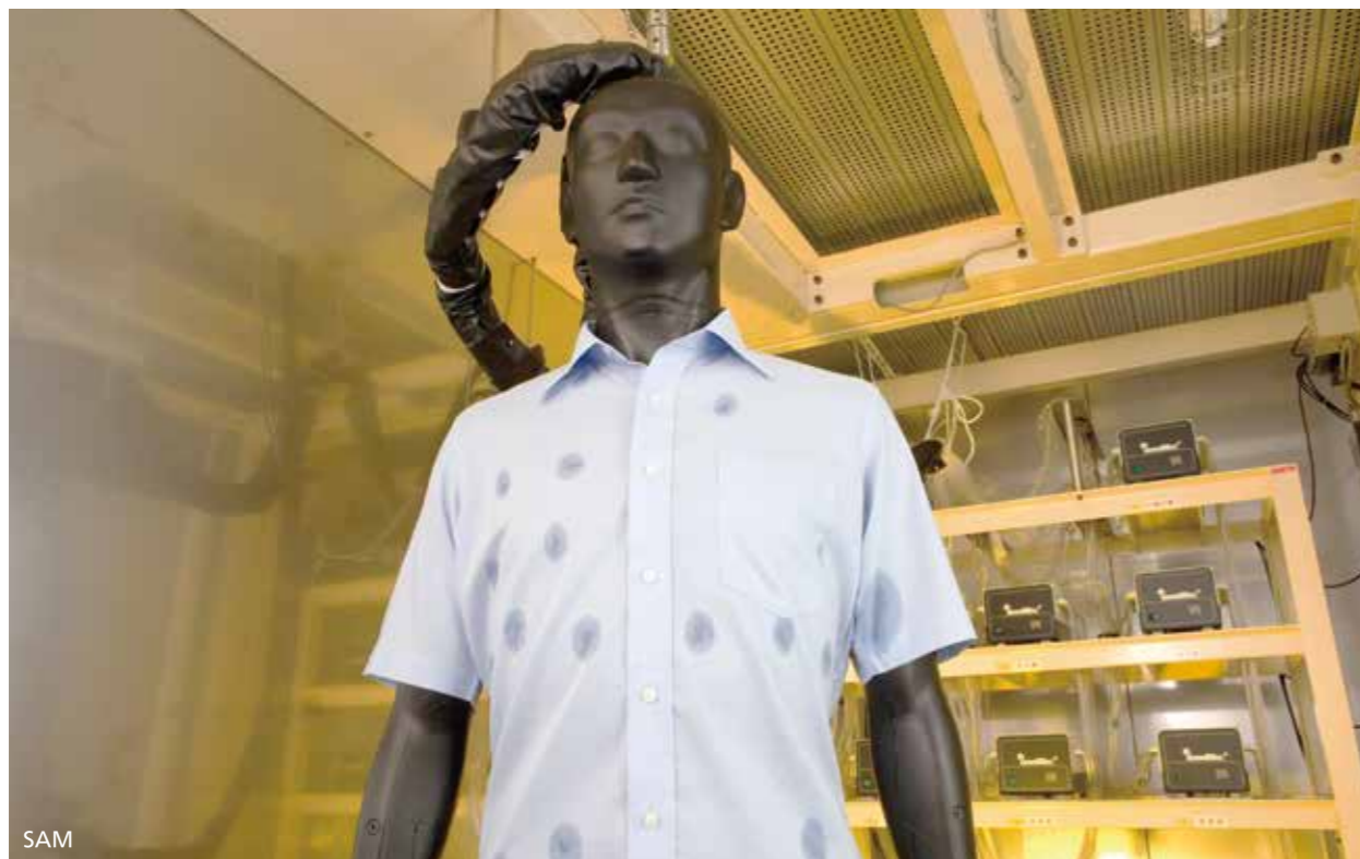
The TOM™ III has more than 200,000 sweating holes on its surface, and can measure temperature and humidity within clothing.
