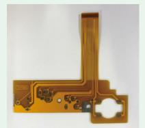
Circuit board using HARDLEN®
