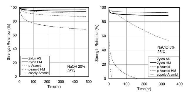
At higher temperatures, the strength of ZYLON® AS staple fiber decreases in acid and also in alkaline.
