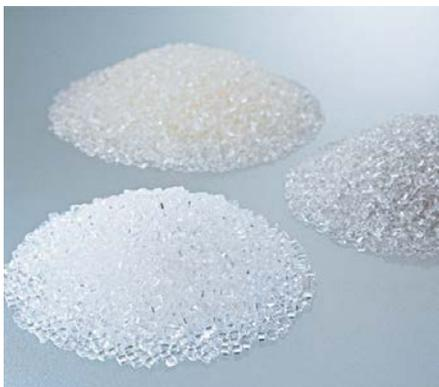
TOYOBO GS Catalyst® (front) enables synthesis of resins with higher transparency than other catalysts
