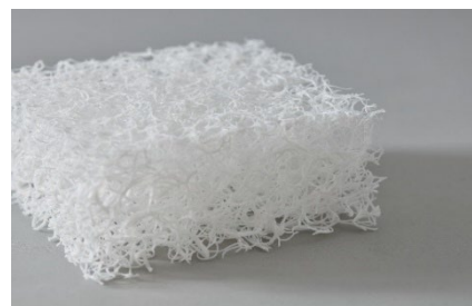
BREATHAIR®, a three-dimensional network structured fiber material
