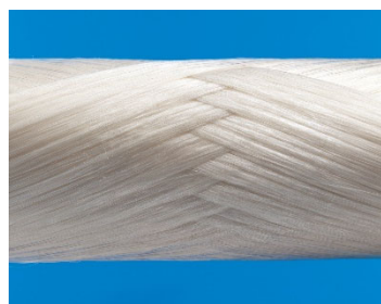
Cross winding structure
