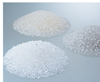
PET resin produced using the TOYOBO GS Catalyst ® (left, front)
