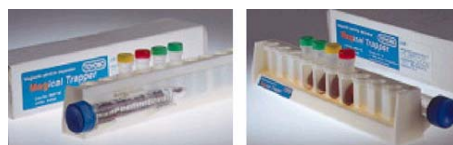
Fig. 2. Magnetic stand Magical Trapper (Code No.MGS-101)
